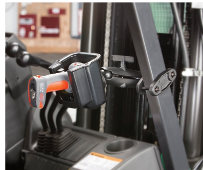
Square Post Clamp, pg. 12 Socket Arm, pg. 20 Device Adapter, pg. 22 Scanner Gun Holder, pg. 26
